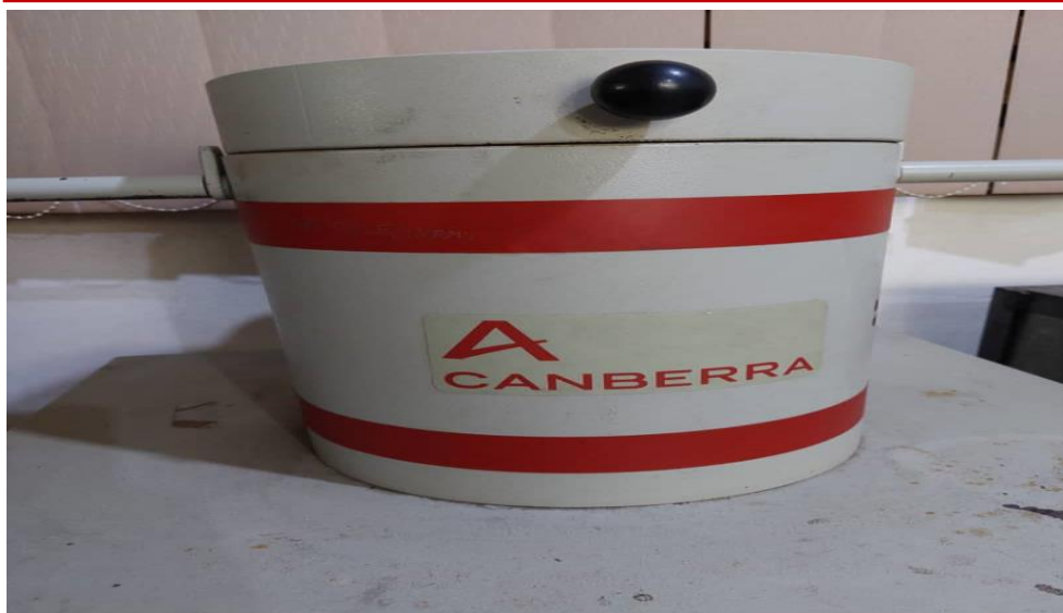
Figure 1: A lead-shielded 76 x 76 mm NaI (TI) detector crystal (Model No.802 series, Canberra Inc. coupled to a Canberra series multichannel Analyzer (MCA) (Model N0.1104) through a preamplifier. Source: NIRPR, University of Ibadan, Ibadan, Nigeria (2025).
