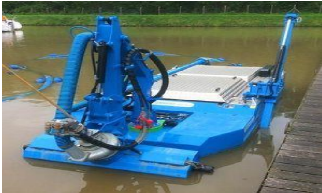
Fig 2: A hydraulic Dredger adopted (from Oliver et al., 2013)
