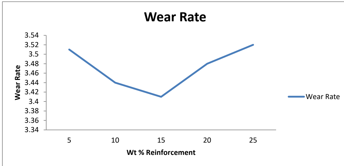
Fig. 3.2: Variation of Wear Rate with Weight Percent of Plantain Peels
